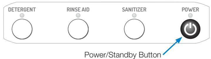
Please note that pressing the Power button **does not isolate the dispenser from line voltage** and therefore, precautions still must be taken to avoid shock when working inside the cabinet.
