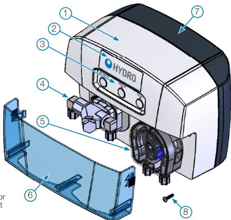
**NOTE:** The Main Cabinet Cover is only available for peristaltic pump configurations and will not be installed on units that use a solenoid.
