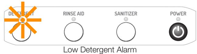
Condition: **Low Detergent Alarm Lockout** (Probe Mode Only)
